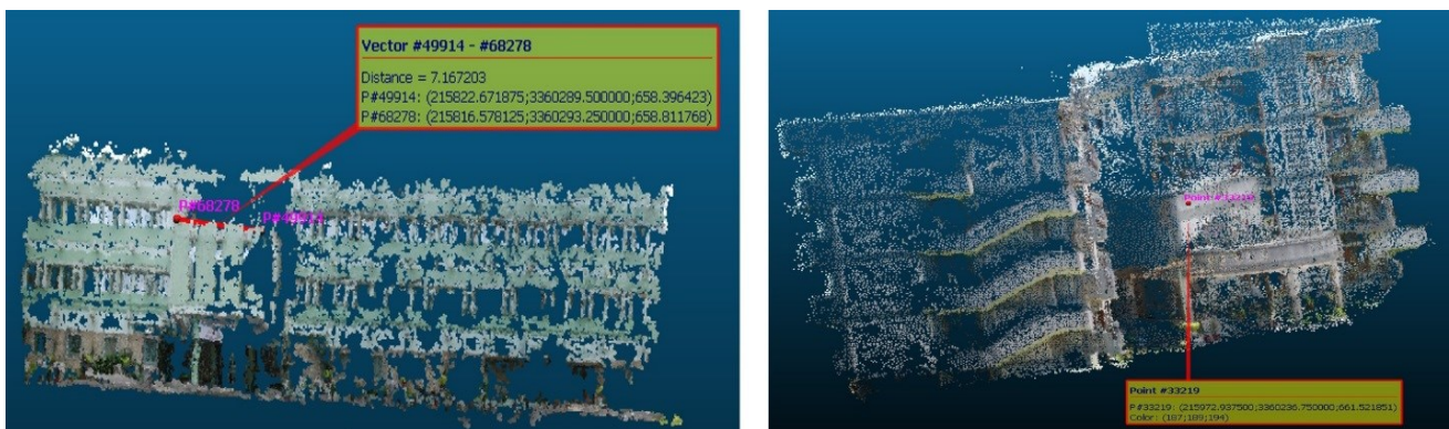
Figure 5. Georeferenced point cloud of Building 1 and Building 2
