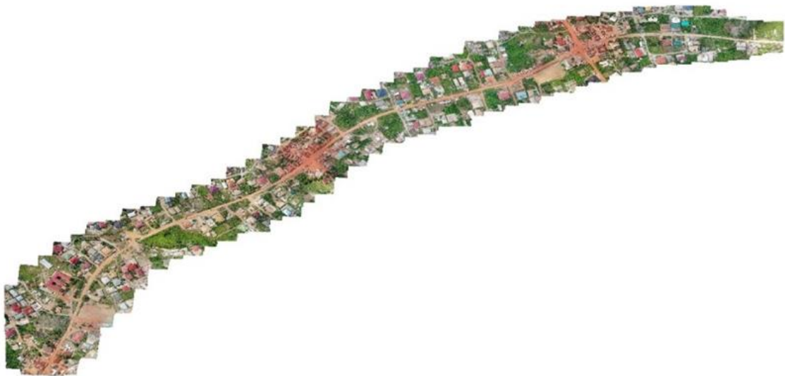
Figure Error! No text of specified style in document.. Orthomosaic obtained from processing the data from the Aerial Survey
