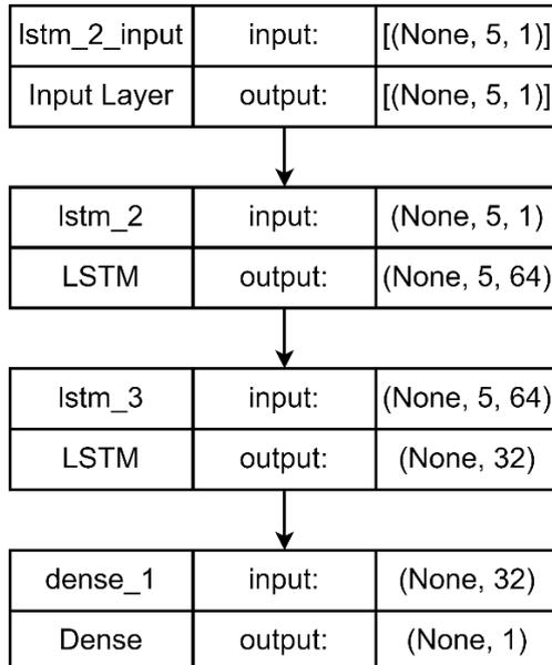
Figure 6. Developed LSTM model architecture
