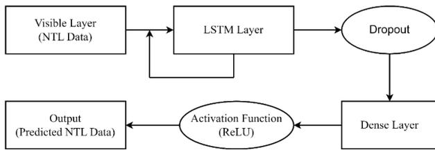
Figure 5. Process flow of developed LSTM model
